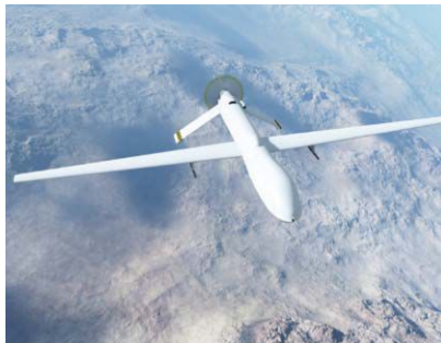
▲ GEODETICS Geo-iNAV provides precise relative position and orientation for UAVs and other platforms.
