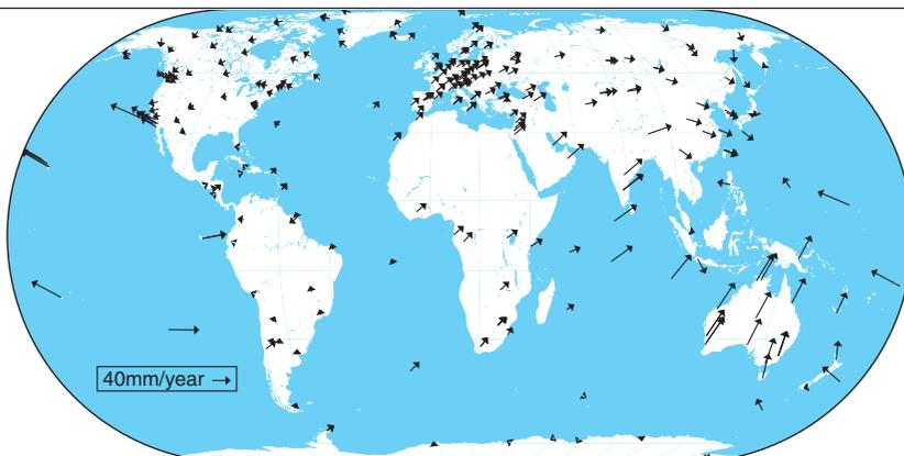
▲ **FIGURE 3** Calculated velocities of IGS stations from a recent weekly update of the IGS cumulative reference frame product. The velocities reflect the movement and deformation of the Earth's tectonic plates.
