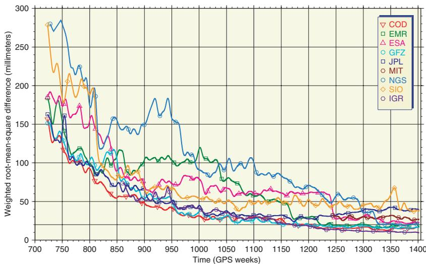
▲ **FIGURE 2** The consistency of the individual analysis centers' satellite orbit solutions has improved over the years to approximately 2 centimeters today. Each trace shows one analysis center as compared to the weighted mean. Graph courtesy G. Gendt, GFZ.
